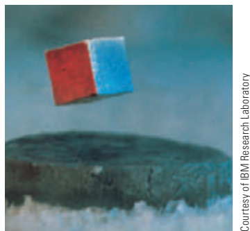
A small permanent magnet levitated above a disk of the superconductor \text{YBa}_2\text{Cu}_3\text{O}_7 , which is in liquid nitrogen at 77 K.
