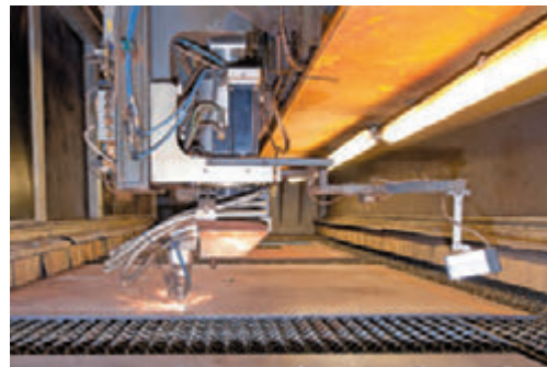
Figure 42.31 This robot carrying laser scissors, which can cut up to 50 layers of fabric at a time, is one of the many applications of laser technology.
