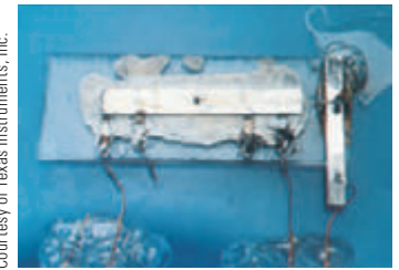
Figure 43.32 Jack Kilby’s first integrated circuit, tested on September 12, 1958.
