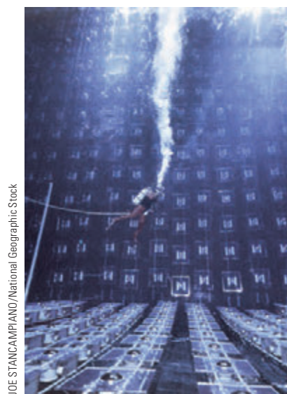
Figure 46.6 (Example 46.2) A diver swims through ultrapure water in the Irvine–Michigan–Brookhaven neutrino detector. This detector holds almost 7 000 metric tons of water and is lined with over 2 000 photomultiplier tubes, many of which are visible in the photograph.
