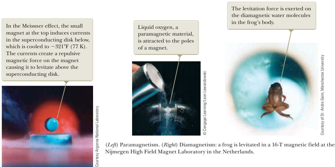
Figure 30.27 An illustration of the Meissner effect, shown by this magnet suspended above a cooled ceramic superconductor disk, has become our most visual image of high-temperature superconductivity. Superconductivity is the loss of all resistance to electrical current and is a key to more-efficient energy use.
