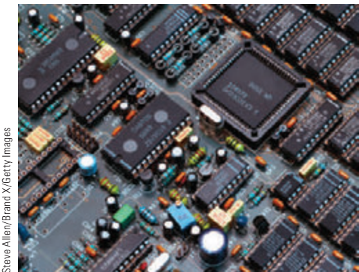
Figure 43.33 Integrated circuits are prevalent in many electronic devices. All the flat circuit elements with black-topped surfaces in this photograph are integrated circuits.
