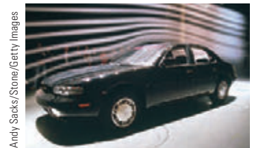
Figure 14.13 Laminar flow around an automobile in a test wind tunnel.
